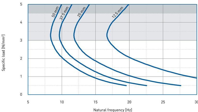
Natural frequency of a single-degree-of-freedom system consisting of a fixed mass and an elastic bearing consisting of PURASYS **vibradyn** HL 3000 on a stiff subgrade.
