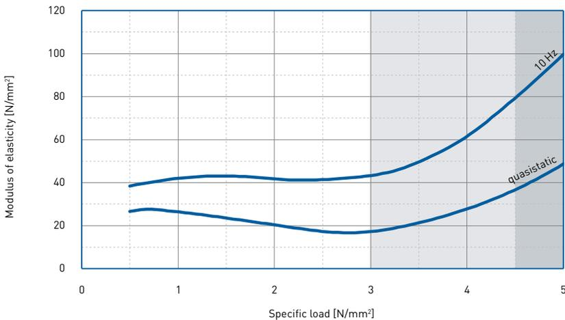
Dynamic test: sinusoidal excitation with an oscillating range of  $\pm 0.11 \text{ mm}$  at 10 Hz
