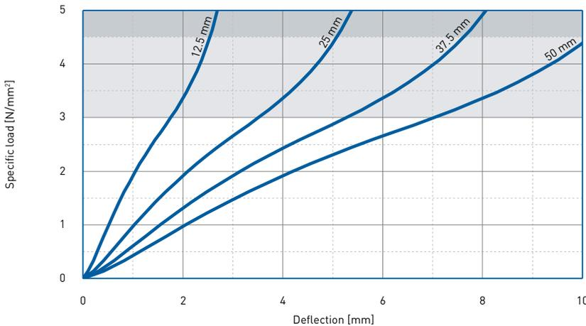
Recording of the 3rd loading; testing between steel plates with emery cloth of granulation K 120 at room temperature measured at  $v = 0.2 \text{ N/mm}^2 / \text{sec}$
